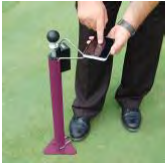
Figure 10: Using the Trufirm with the bluetooth ap and an iPhone
